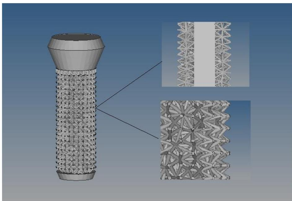
Figure 7: Implant structure after optimization
