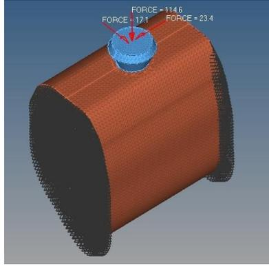
Figure 3: Applied loads and boundary conditions of FEM model.
