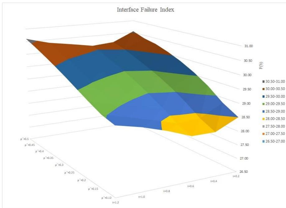
Figure 5: The effect of relative density and implant interface thickness at interface failure index.
