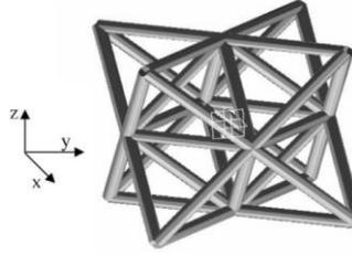
Figure 4: Structure of a unit cell of the regular octet-truss lattice material[22].
