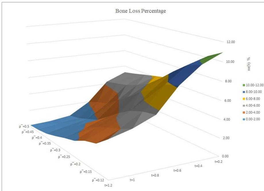
Figure 6: The effect of relative density and implant interface thickness at bone loss percentage.
