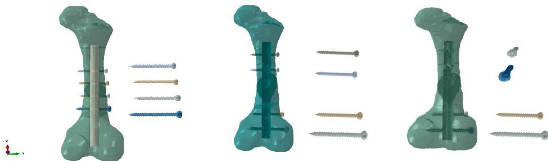
184 Figure 3: A) 1 st condition ( BLK1 ) four lateromedial direction cortical screws. B) 2 nd 185 condition ( BLK2 ) four lateromedial direction cortical screws, two at 186 proximal diaphysis and two at distal condylar region. C) 3 rd condition 187 ( BLK3 ) two lateromedial direction at distal condylar region and two 188 caudocranial direction at proximal diaphysis. 189
