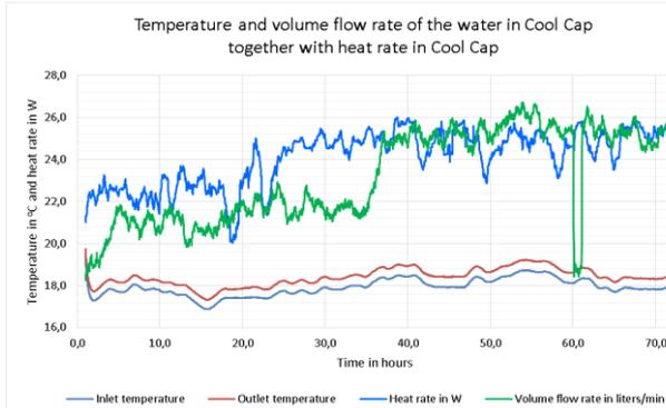
Figure 11: Measured temperatures and volume flow rate of the water in Cool Cap together with heat rate in Cool Cap – patient N1
