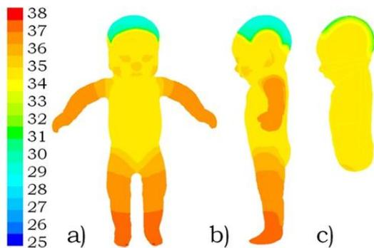
Figure 7: The temperature distribution (in °C) on the skin surface (a), at the left side (b) and on the central cross section (c) at the end of the cooling stage.
