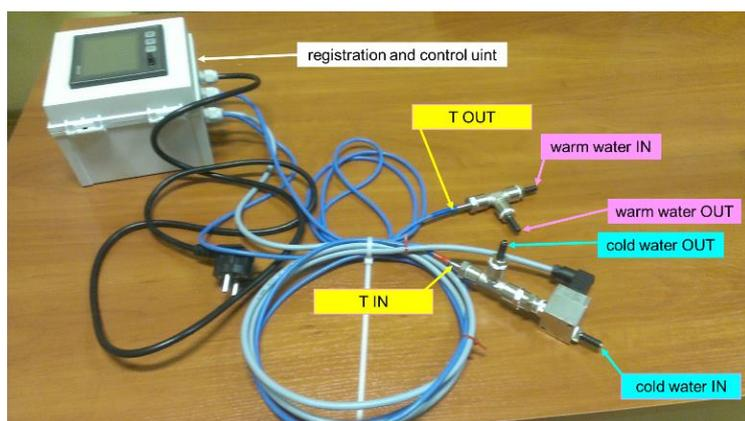
Figure 8: The water flow meter equipped with temperature sensors to monitor fluctuations of heat flux in the brain cooling process remotely
