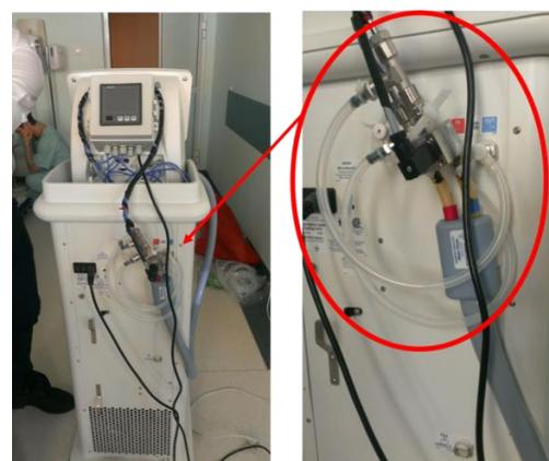
Figure 9: Cool Cap equipped with the water flow meter and temperature sensors
