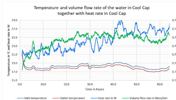
Figure 15: Measured temperatures and volume flow rate of the water in Cool Cap together with heat rate in Cool Cap – patient N3
