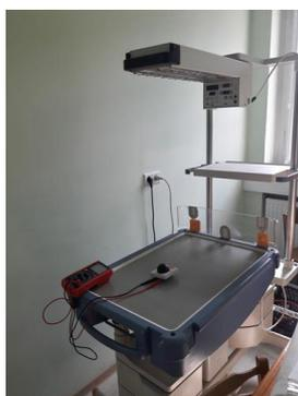
Figure 10: Globe thermometer measuring radiative temperature
