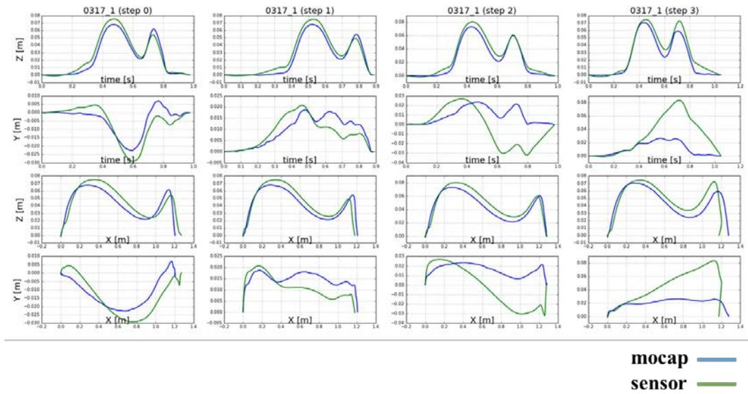
Figure 5: Comparison of the measured (motion capture) and estimated (sensor) trajectories
