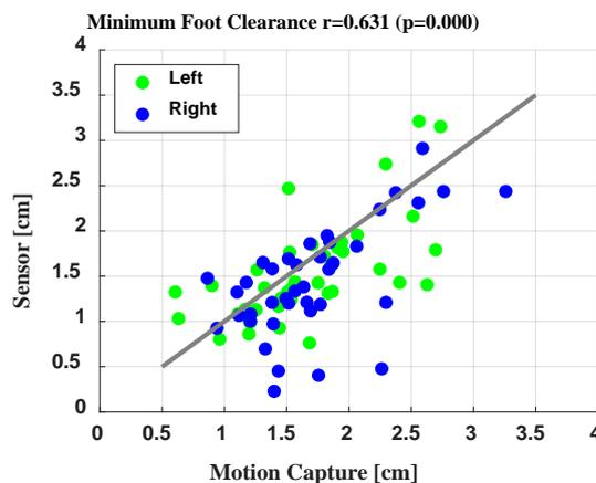
Figure 4: Agreement between motion capture and sensor-estimated MFC
